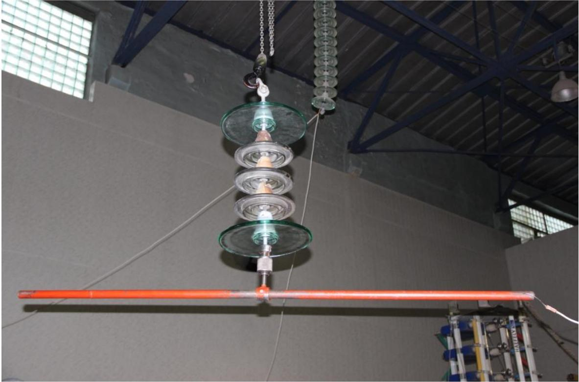
**Fig. 4 New configuration string insulator unit test (wet).**
